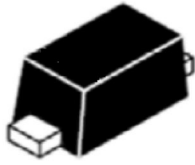
SOD-523 (Top View)
